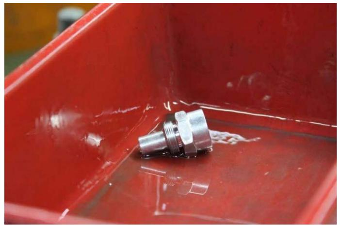
Fresh out of the thread rollers, this fitting is nearly ready to be put into inventory and shipped wherever customer demand says that it must go. Hours before this was just another piece of bar stock on the materials rack. Pretty awesome.
