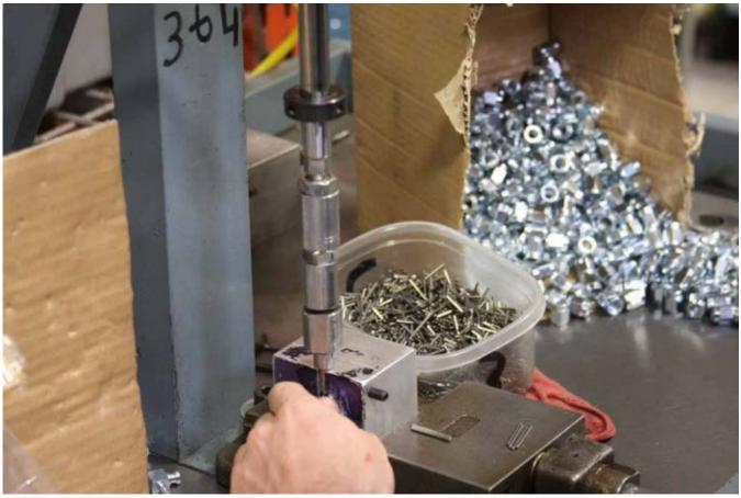
At this work station the pins were being inserted into the Fragola manufactured nuts with a pneumatic ram. You can see the pile of nuts in the background, a couple of pins on the station and the fixture that aligns everything as well.
