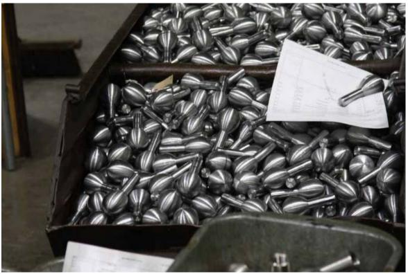
These pieces are known as lollipops and they are what a rod end starts life as. Technically the rod end starts life as a long piece of steel in a screw machine but you get where we're going with this. The flats are machined into the bulbed end and they really start to take shape.
