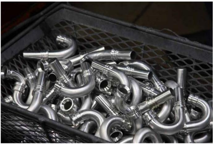
We stood for a while and watched the little mandrel bender work its magic on these bad boys and just admired how pretty and clean they were. Mandrel bending means no pinching, no loss of flow, and no performance issues. It isn't the cheapest way to do it but it is the best. A hallmark of the company.
