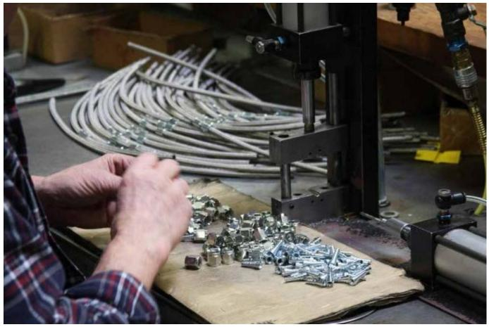
The company's pre-assembled hoses are a big seller and here we see a work station where some hoses are being assembled. There is a lot of hand work in this process and it really is interesting to watch. This guy was moving like lightning.
