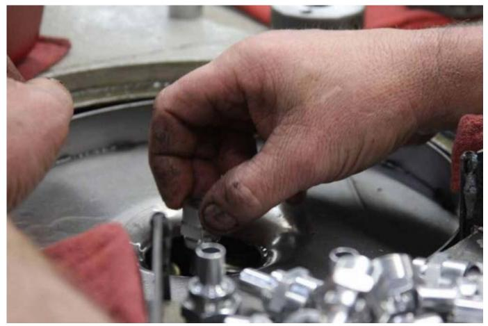
Here's a fitting about to be dropped into a thread rolling machine. The guys who have been doing this for years are lightning fast at it and while one hand is dropping the other has another fitting to chase this one into the machine. The rolled threads are stronger than cut threads by a ton.
